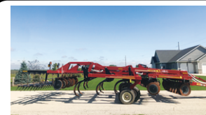
2014 MCFARLANE QT209 DEMO UNIT, FULL WARRANTY, 9 SHANK, REAR DISK LEVELER, REAR 5 BAR SPIKE DRAG
