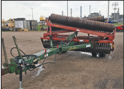
Brillion Pulverizer X-Fold; 34' working width, Notched Ductile Rolls, Scrapers, 11L-15 Duals. E40005 . . . . . $15,374
