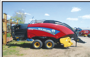
NEW New Holland 330P Big Square Baler 35.4 x 31.5 bale size; packer cutter; autosteer tandem axle; wh500/50-17.0-14pr alliance; 1 3/4" 20 spline; folding hyd roller chute; color monitor manual jack; caster pick up wheel . . . E38708
