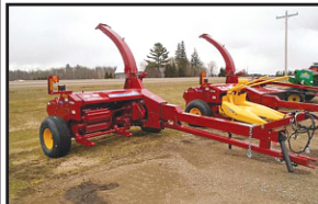
NEW New Holland FP240 Forage Harvester metal; single axle; 1 3/8" 21 spline; automatic hydraulic hitch . . . . . E38467
