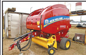
NEW New Holland Roll Belt 460 Round Baler 4x6; rotor cutter; endless belt; deluxe wrap; net only; 540 rpm with cut out clutch; ties: 18-16.1st; heavy duty density system; bale ramp; 2.07 pickup; 15 x 16.00-6 casting; manual hyd pickup lift; 5 bar pickup reel; drop floor; manual rotor reverser; 2.07m roller wingguard; pto sprt locking pin. . . . . E38707
