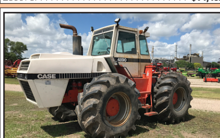
Case Tractor 4890; 4WD, Crab Steer, 12F/4R P.S., CHA, 6 Cyl, Turbo, 300HP, 3Pt, Top Link, Ock Hitch, 4 Remotes, Big 1000 pto, 30.5L-32. E39195 . . . . . $14,999
