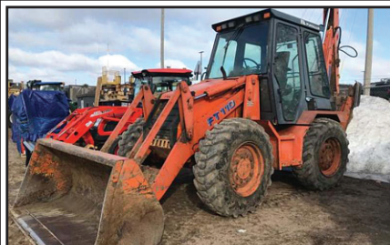
Fiat Allis TLB FT110; 4wd, CHA, Radio, Blk Heater, Joystick, 105hp, 8 Spd Shuttle, 38" Backhoe Bkt, 6 Teeth, Extend-a-hoe, Rear Rmts, 8" Frt Pin On Bkt, Aprox 21850lb machine, 15.5-25 tires. E40002 . . . . . $16,999
