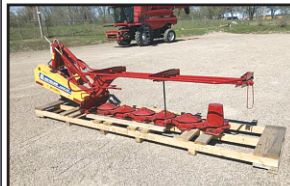
NEW New Holland 108M Discmower cat II; 7'10" cutting width; 6 pods; 540 PTO; 3 pt mount. . . . . E39472
