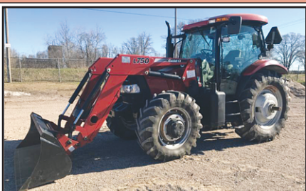
Case IH Tractor Maxxum 140 Pro; CHA, MFWD, Dlx Cab, 540/1000 pto, 3Pt Top Link, Two Rmts, Blk Htr, 6cyl Turbo, 139Hp, 17F/16R Partial P.S. Left Hand Reverser, L750 Loader, 7" Euro Mt Bkt, 18.4R38. E40112 . . . . . CALL
