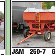
J&M 250-7 GRAVITY BOX WITH WOOD SIDE EXTENSIONS , mounted on a Kory 6872 running gear with used truck tires ..... $895
