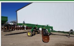
'04 JD 670, 20'4" Disk, 11" Spacing, Hyd Adj Hitch, Self Adj Scrprs. . . . . $13,900
