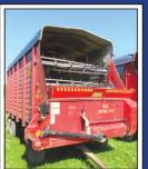
SED H&S 7+4 Forage Box, 16' Long, Right Hand Apron Unload, Knowles 10 Ton Tandem Axle Gear, 12.5L-15 Tires w/ 6 Bolt Rims #BX7348
