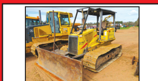
2001 New Holland DC80 LGP Dozer , Open ROPS w/ canopy, 24" pads, good U/C, 118" six way blade, rear hitch, block heater, front & rear work lights, hydrostatic drive w/ hi-lo transmission, 84 HP, 16,711 lbs. .... $20,995
