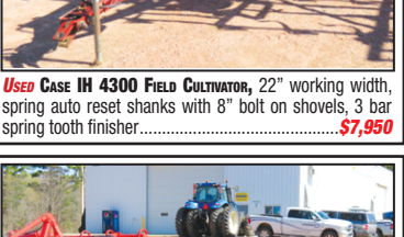
USED CASE IH 4300 FIELD CULTIVATOR , 22" working width, spring auto reset shanks with 8" bolt on shovels, 3 bar spring tooth finisher..... $7,950
