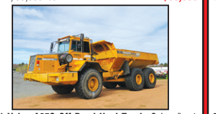
2001 Volvo A35C Off Road Haul Truck , Cab w/heat, 26.5R25 tires, 6x6, plastic dump box liner, 19 cubic yd cap., heated air ride seat, no tailgate, 351 HP Volvo diesel, 56,659 lbs. .... $65,000
