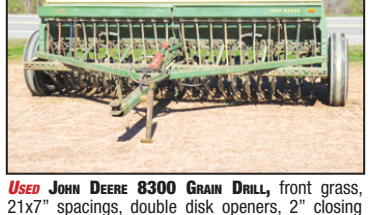
USED JOHN DEERE 8300 GRAIN DRILL , front grass, 21x7" spacings, double disk openers, 2" closing wheels, rear walk board, rear hitch, 7.50-20 marker tires, cylinder and hoses ..... $4,950
