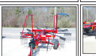
NEW NEW HOLLAND PR 3114 ROTARY RAKE , 9'8" raking width; 6'7" transport width; hyd lift; single rotor with 11 raking arms; 4 double tooth tines per arm; deflector curtain..... CALL
