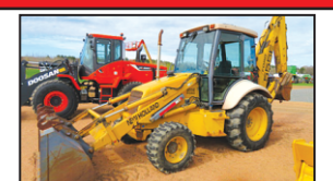
1996 Ford/New Holland 555E Loader Backhoe , Cab w/heat, extend-a-hoe, 4WD, 16.9-28 rear tires, 14x17.5 front tires, 88" front bucket, 24" backhoe bucket w/ teeth, 4 speed, 79 HP, 14,010 lbs. .... $22,495
