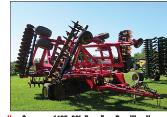
Used SUNFLOWER 1435 30' ROCK FLEX DISK WITH HYDRAULIC SELF-LEVELING, 21 1/2" front disc blades, 22 1/2" rear disc blades, rear hitch and light plug, light kit, scraper kit..... $29,500
