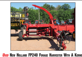
Used NEW HOLLAND FP240 FORAGE HARVESTER WITH A KERNEL PROCESSOR, Metal III, hydraulic swing hitch, hydraulic spout rotation, electric deflector, lights, tandem axles with 11L-15 tires, rear hydraulic hitch, 1 3/4" PTO, 6 knives and shear bar..... $18,900
