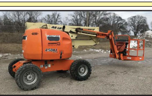
JLG Boom 450AJ Lift; Articulating boom lift, Dual Fuel, 45ft boom, Hydraulic rotation and leveling, 4x4, Gas, Block Htr, 500lb Cap, 24'5" Reach, 16145lb Machine. 33x15.50-16.5 E39785. .... $29,989
