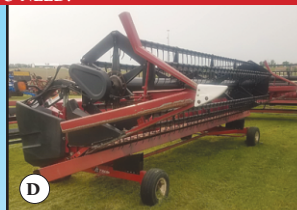
D10 CIH 1020 20' Flex Head , Field Tracker, 1.5" Cut, Long Dividers, Hyd Fore and Aft..... $8,500
