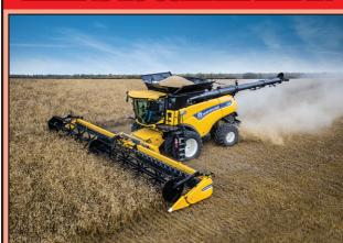
w - New Holland CR7.90 Combine: IntelliSense combine automation, corn/bean, 40 KPH max road speed, front differential lock, 2 speed powered rear axle, IF1250/50R32 front single tires, IF850/60R26 rear tires, axle extensions, platform extension, heated floor mat, leather operator seat, satellite radio, variable speed high nower feeder drive with dynamic feed roll, abrasive wear elevator with grain cam, in cab electric folding A503
