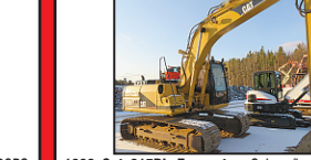
1998 Cat 315BL Excavator, Cab w/heat, 27.6" wide pads, very good U/C, Aux. hydraulics (1 way flow only) NPK auto lube unit, Cat hyd. pin-grabbing Q/C, 46" bucket w/6 teeth, work lights, 99 HP, 38,200 lbs..... $41,200
