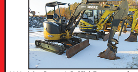
2013 John Deere 35D Mini-Excavator, Open ROPS, 68" dozer blade, 12" tracks, 2 speed, mechanical Q/C with 12", 18" and 30" buckets, aux. hydraulics, 28.6 HP Yanmar diesel, 7,760lbs..... $25,995
