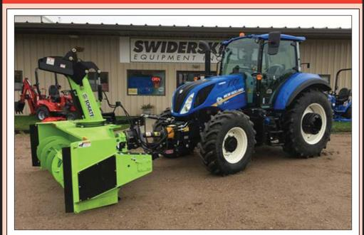
**NEW NH T5.120 TRACTOR;** MFWD; Cab W/ AC; 16X16 SPS Transmission; 40 KPH; 3 Mid Mount Valves; Loader Ready; 14.9R24 Front Tires; 460-85R34 Rear Tires D09499
