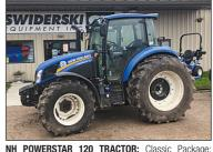
NH POWERSTAR 120 TRACTOR; Classic W/ 12X12 Transmission Reverser; MFWD; 2 Rear Remotes; 540/1000 PTO; 4 X110 LB Rear Wheel Weights; 8 Front Suit Case Reverser; MFWD; 2 Rear Hemoles, 540/1000 1.0, 4 X110 LB Rear Wheel Weights; 8 Front Suit Case Weights; Front Fenders; 380/85R24 Front Fenders; 460/85R34 Rear Tires; One Owner Tractor With Under 250 Hours; Warranty Remaining Until 4/18/21
