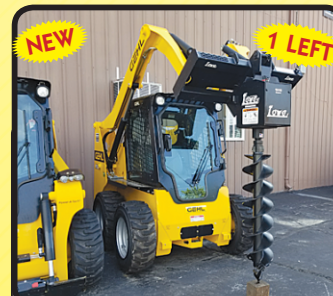
LOWE 1650 POST HOLE AUGER, W/ 12" BIT
