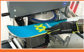
Our 3D Ceramic Disc Grinder can restore the proper edge profiles and correct bevel angles on any ski.
