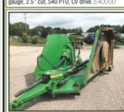
Hyd lift, Hyd Fold Wings, Small 1000 pto, Solid Laminate Tires, 4 on Main Frame, 2 per/wing.
