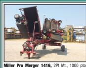
Hyd Resevoir and pump, Each Wing Independent Merge to Right, Merge Both to Center, Merge Both Out, Aprox Two Seven Ft P/up Heads, Lights One Year Old Belts. 11L-15. Nice Local Trade!
