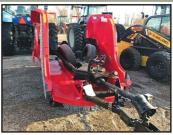
♥ Woods BW15.50 Batwing Dual-wing **Rotary cutter** 15 ft, STD Duty, 45-200 hp, 10 gauge, 2.5" cut, 540 PTO, CV drive. *E40000*
