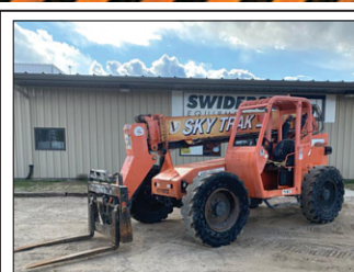
SKYTRAK 6034 TELEHANDLER ; Cummins 74 HP Engine; Left Hand Reverser; 6000LB Lift; 36" Lift Height; 22' Max Reach; 3 Way Steering; Hydraulic Coupler; 48" Forks; Block Heater; 13.00-24 Solid Rubber Tires D10240 ..... $26,900
