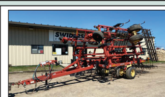
KRAUSE 5635-24 FIELD CULTIVATOR ; 24' Width; 3 Section Folding; Swivel Caster Wheels; 5 Bar Spike Tooth Harrow; Road Lights; Walking Tandem; 11L-15FI Tires D10311 ..... $17,995
