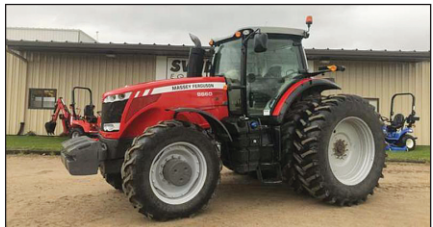
MF 8660 TRACTOR , MFWD, Front Suspension, CVT Transmission, 50KPH, Active Seat Suspension, 540/1000 PTO, 46 GPM Pump, 5 Rear Remotes (3 Fingertip, 2 Joystick), Power Beyond, Engine Block Heater, 2 Beacons, Front & Rear Work Lights, 24 Front Weights, Wheel Weights, Front 480/70R34 Tires, Rear 520/85R46 Duals, Powertrain Warranty Until 6/12/2020 or 2633 total machine hours, DX9790 ..... $99,995
