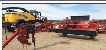
NEW HOLLAND H7560 CENTER PIVOT DISCBINE ; 15' 7" Cutting Width; Flail Conditioner; 1000 PTO; Road Lights; 31X13.50-15 Float Tires D10254 ..... $14,995
