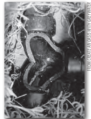
Cutaway view of flow-splitter; a fitting that is largely self-cleaning with no filtration.
