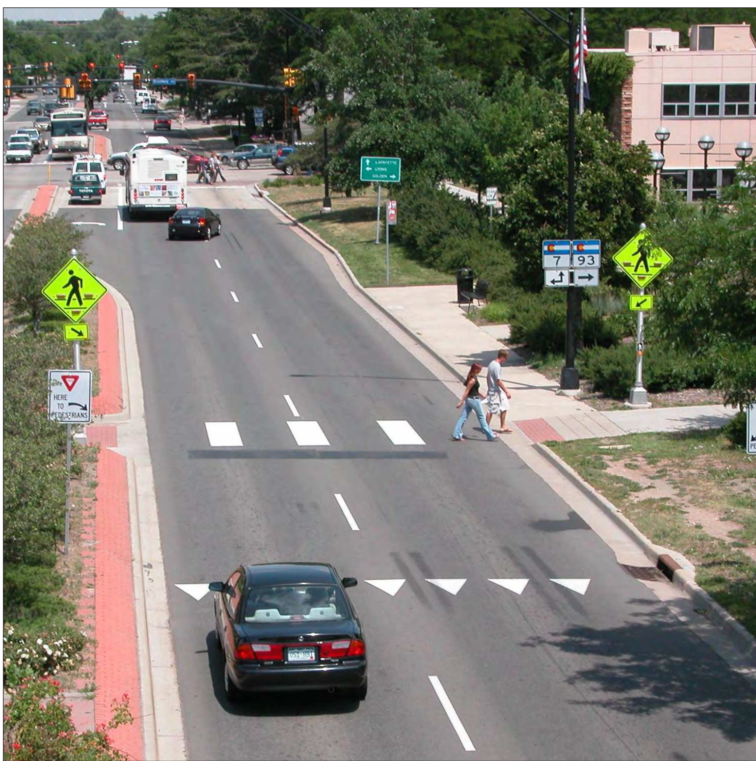
Example of a high visibility pedestrian crossing with RRFBs.
