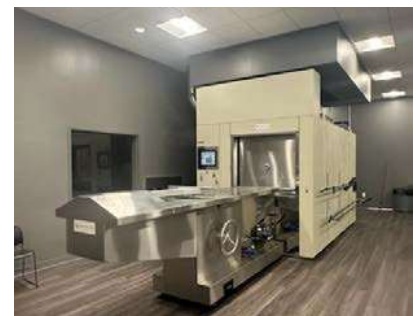
FT III Cremator On Site
