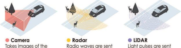
Light pulses are sent out and reflected off objects. Can define lines on the road and works in the dark.
