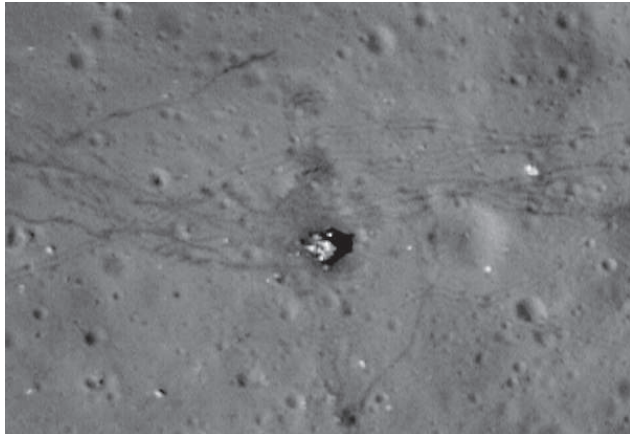
The Apollo 17 Lunar Module “Challenger” descent stage is shown. Notice the tracks from the lunar rover around it.
