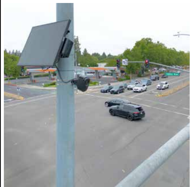
One of Pleasanton's 35 Flock Safety cameras, attached to the light post in the foreground, records the license plates of vehicles that come into view, checks them against known hotlists, and stores the photograph for possible later searches. Photo — David Jen
