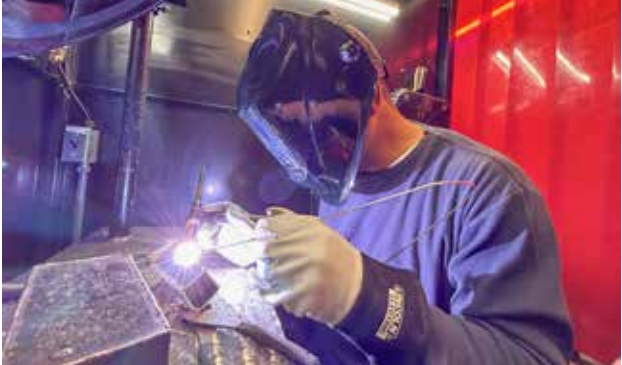
A Las Positas College student uses a process called Gas Tungsten Arc Welding to manually weld together carbon steel components. (Photo — Scott Miner)
