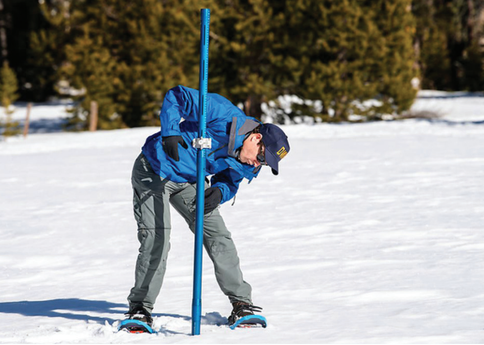
John King, Water Resource Engineer of the California Department of Water Resources Snow Survey Section inserts the long aluminum snow depth survey pole into the snow for the first DWR snow survey of the 2019 season held at Phillips Station in the Sierra Nevada Mountains. The survey site is approximately 90 miles east of Sacramento off Highway 50 in El Dorado County. Photo taken January 3, 2019. (Ken James - Cal. DWR)
