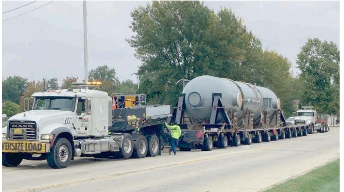
The large gray vessel pictured above, called a slug catcher, was on its way through Herscher to the Kinder Morgan Natural Gas Pipeline. During the winter months when natural gas is withdrawn from the Mt. Simon aquifer, the slug catcher separates the free water and sand from the gas stream in order to protect downstream equipment and provide clean, dry natural gas. The slug catcher is now in its new location south of Herscher.
