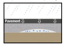
1. Water leaks into pavement from snow, ice and 2. The frozen water melts, weakening the rain. The surface cracks when the water freezes. roadway.
