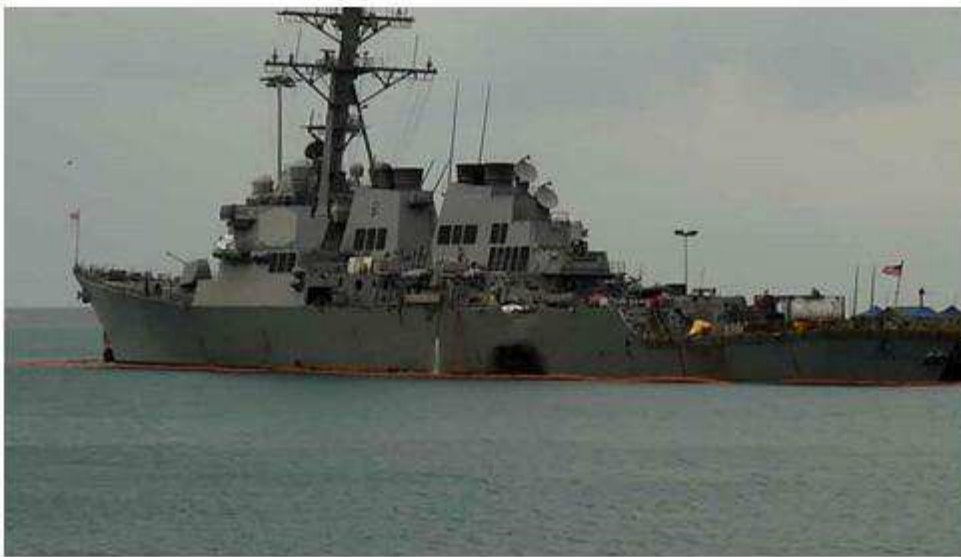
Figure 19 – Port side of JOHN S MCCAIN post-collision
