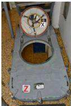
Figure 12 – Primary egress from Berthing 5 Left: from within Berthing 5 Right: Above on the deck outside Berthing 5
