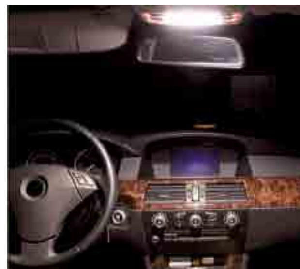
LEDs (top) are brighter and more durable than standard incandescent lights (below), and guaranteed to last up to 12 years.
