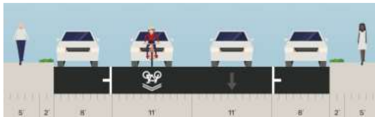
Figure 4 – Typical Existing Cross-Section
