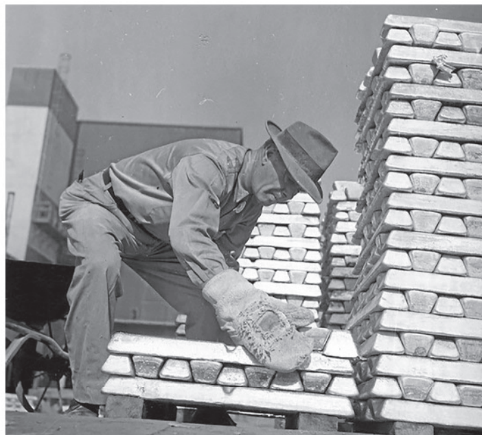
Above: The note accompanying the historical photograph says: "Enormous asbestos mittens must be worn by men handling the thousands of hot magnesium ingots produced daily at Basic Magnesium's giant plant in the Southern Nevada desert. A number of units of this plant are now in production. Full operation is scheduled for the summer of 1943." This photograph was taken by Fritz Henle, according to the Library of Congress. Left: A 1943 aerial view of the Basic Magnesium, Inc. plant site in Gabbs, Nevada. The site is surrounded by the immense Nevadan desert.
