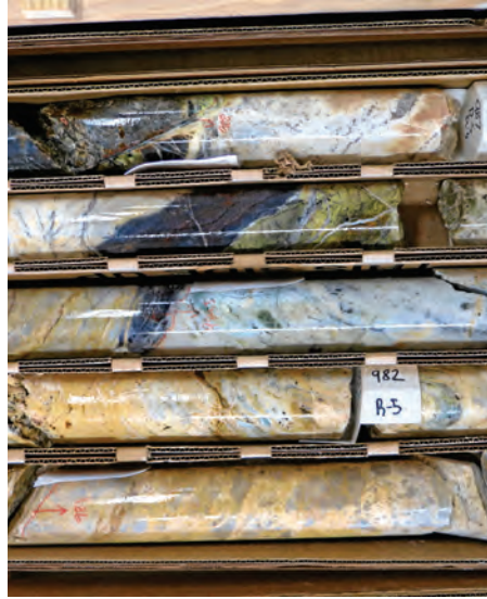
Core samples from American Pacific’s Madison Copper-Gold Project in Montana, taken from Hole C17-24. The samples show the carbonate-latite porphyry contact, displaying chaotic folding and brecciation.
