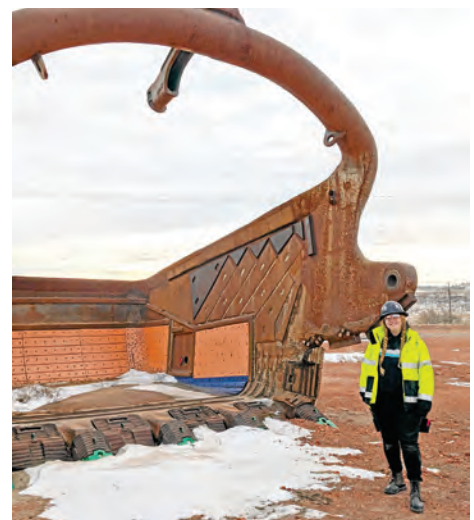
Jess Scanlan stands next to one of the buckets at the Westmoreland Rosebud Mine that can scoop up 75 yards of overburden.
