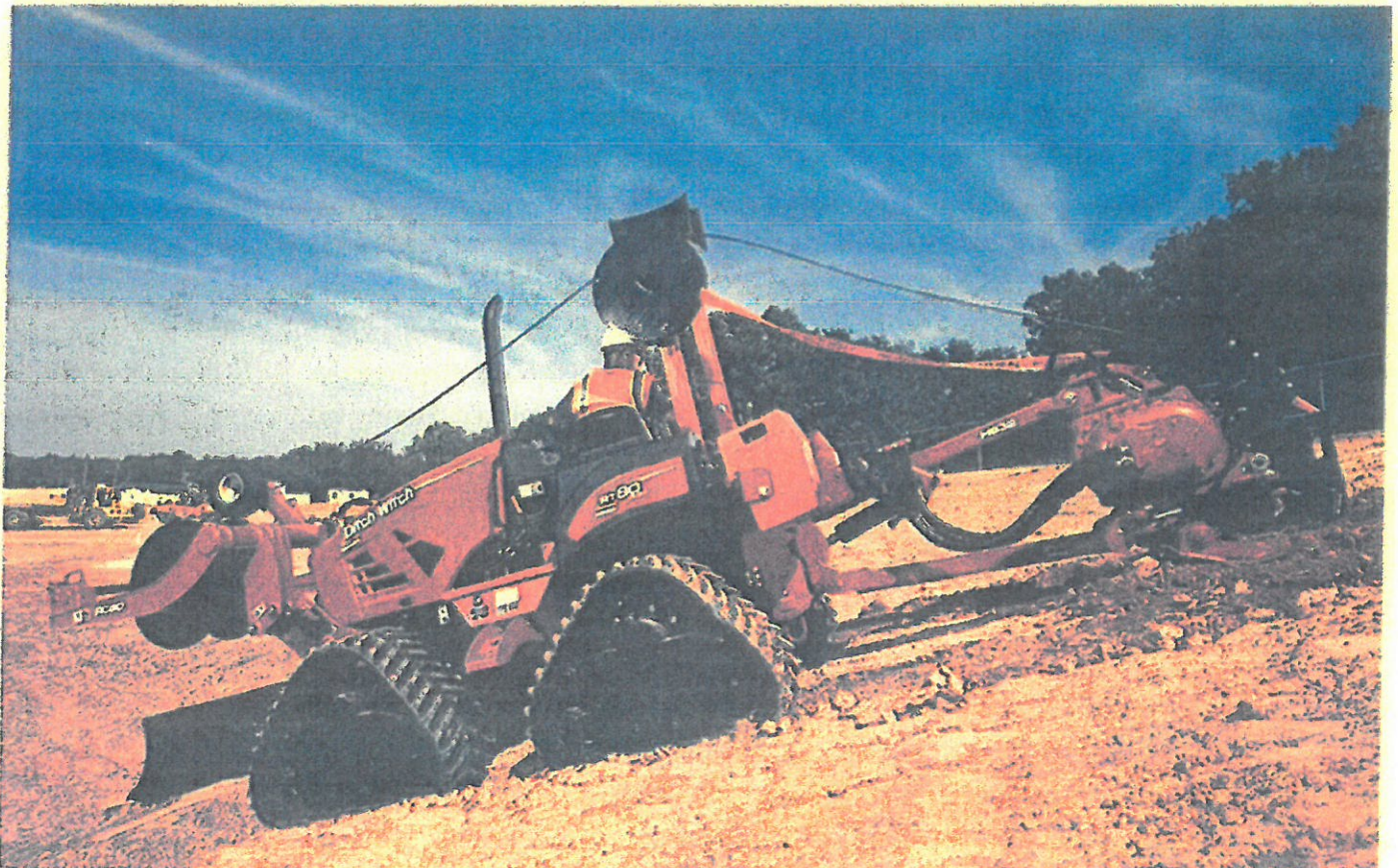
Picture 4. A vibratory plow capable of installing new communication cable
