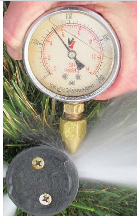
Pictures 4 & 5 Sprinkler head pressure testing during operation. The sprinkler on the left is on hole 5 and has an operational pressure of less than 50 psi. The picture on the right is a sprinkler between the driving range and hole 10, with an operational pressure of 78psi. Optimal operating pressure is 80 psi.
