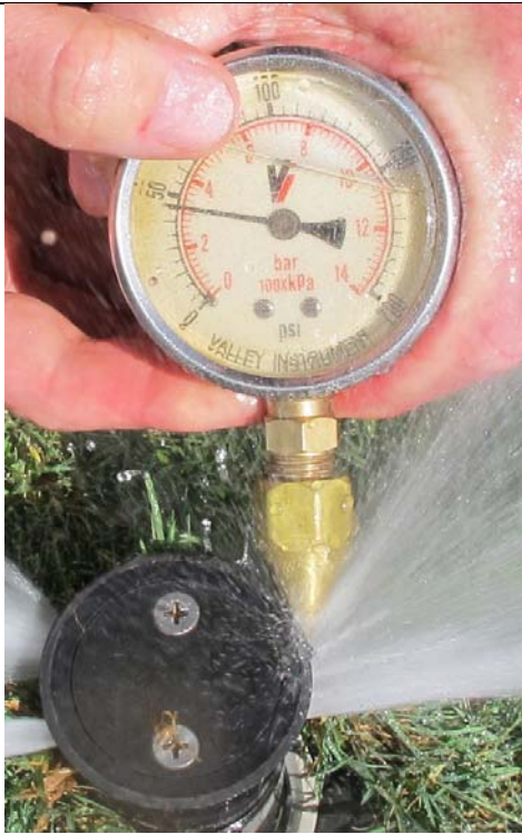
Pictures 4 & 5 Sprinkler head pressure testing during operation. The sprinkler on the left is on hole 5 and has an operational pressure of less than 50 psi. The picture on the right is a sprinkler between the driving range and hole 10, with an operational pressure of 78psi. Optimal operating pressure is 80 psi.
