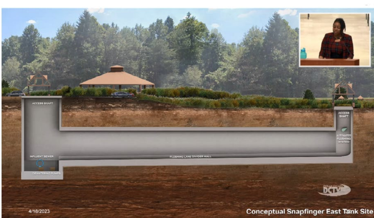
Figure 2: Side View of Below-Grade In-Basin Storage Facility 26
