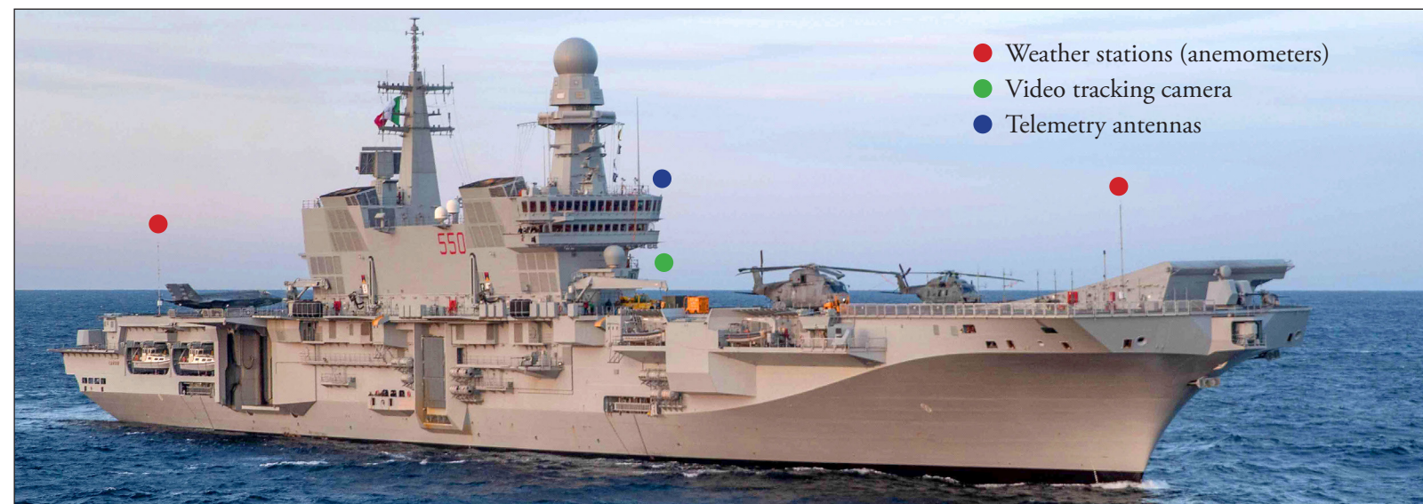
ITS Cavour: ATR instruments gather data from bow to stern for the sea trials. (U.S. Navy photo)
