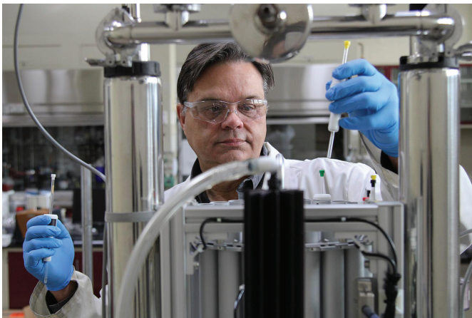
U.S. Army Combat Capabilities Development Command Chemical Biological Center research chemist Dr. Terry Henderson loads an autosampler of a Bruker Nuclear Magnetic Resonance to demonstrate one of several analytical capabilities. NMR spectroscopy is one of several analytical techniques used to determine structural information of a chemical or compound, as well as to determine physiochemical properties. |Gabrielle White, DEVCOM CBC Public Affairs
