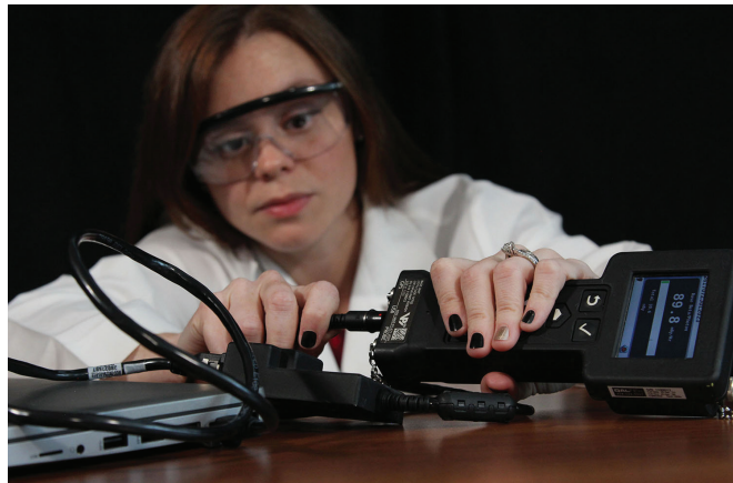
Anamaria Kovalcik, a contractor supporting the Joint Program Executive Office for Chemical, Biological, Radiological, Nuclear Defense, uses the Sensor Network Adaptor to connect a sensor to her laptop. |Gabrielle White, DEVCOM CBC Public Affairs
