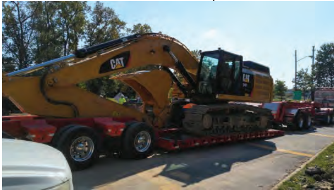
Excavator. Was told had to be on road plates
