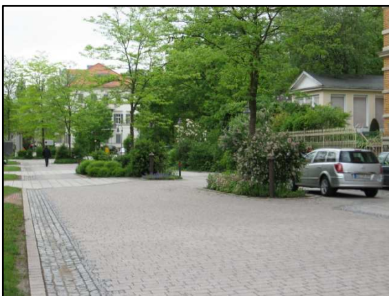
This shared street in Germany lacks sidewalks, but the textured pavement and street trees calm traffic and invite pedestrians to walk in the street.
