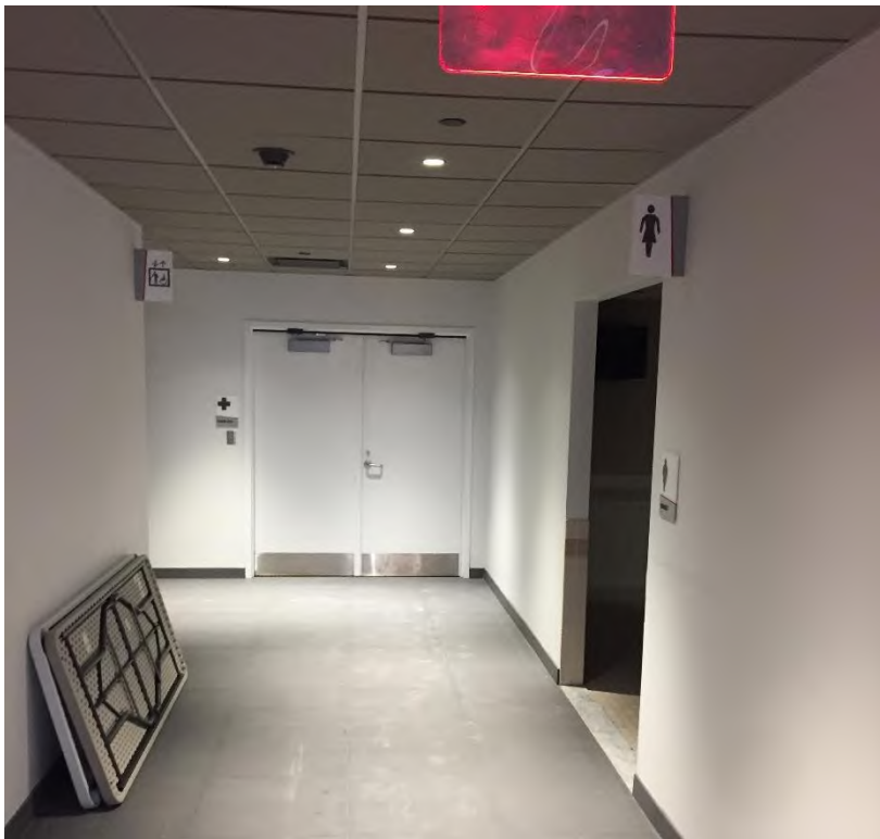
Corridor 231.12: Corridor may potentially be a dead end corridor. Use of medical or security space may have once served as the means of exit. To be further analyzed.
