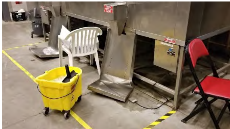
Ice Factory: Ice chutes are damaged from impacts.
