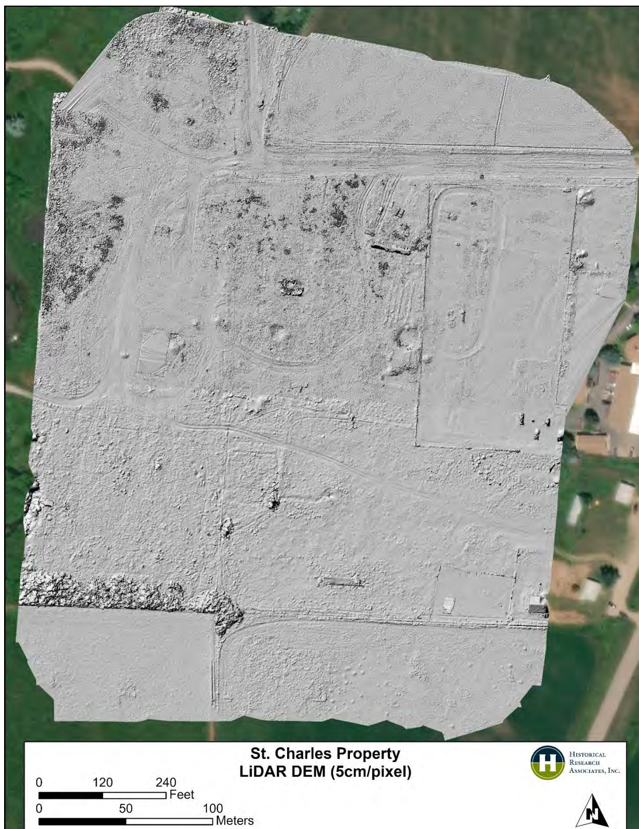
Figure 3. A bare surface topographic model of the St. Charles property with as much vegetation removed as possible.
