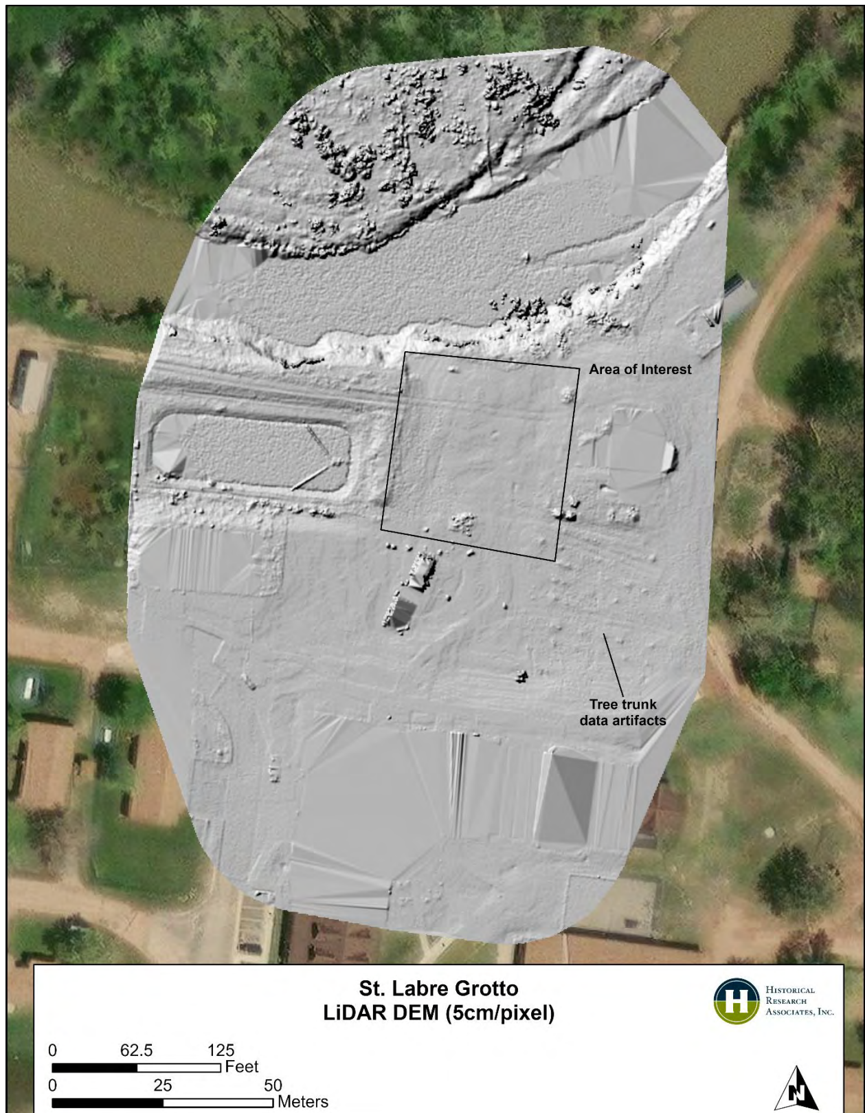
Figure 13. A bare surface topographic model of the St. Labre grotto location, with as much vegetation removed as possible.
