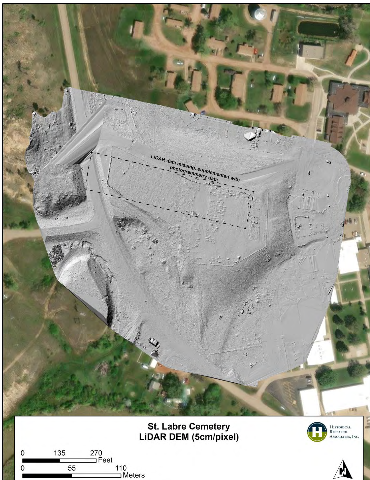
Figure 11. A bare surface topographic model of the St. Labre Mission Cemetery, with as much vegetation removed as possible. Note area where LiDAR data was not collected.
