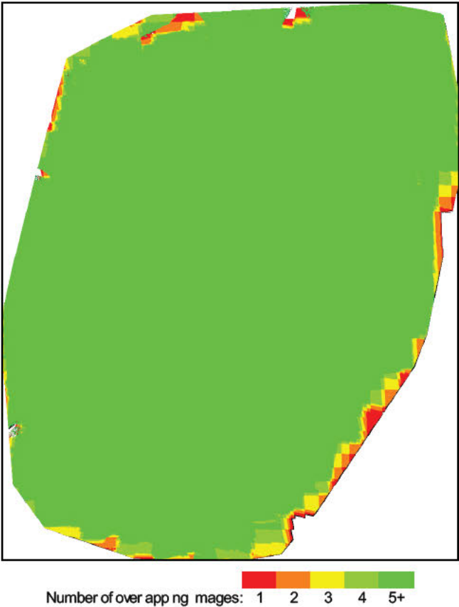
Figure 4: Number of overlapping images computed for each pixel of the orthomosaic. Red and yellow areas indicate low overlap for which poor results may be generated. Green areas indicate an overlap of over 5 images for every pixel. Good quality results will be generated as long as the number of keypoint matches is also sufficient for these areas (see Figure 5 for keypoint matches).
