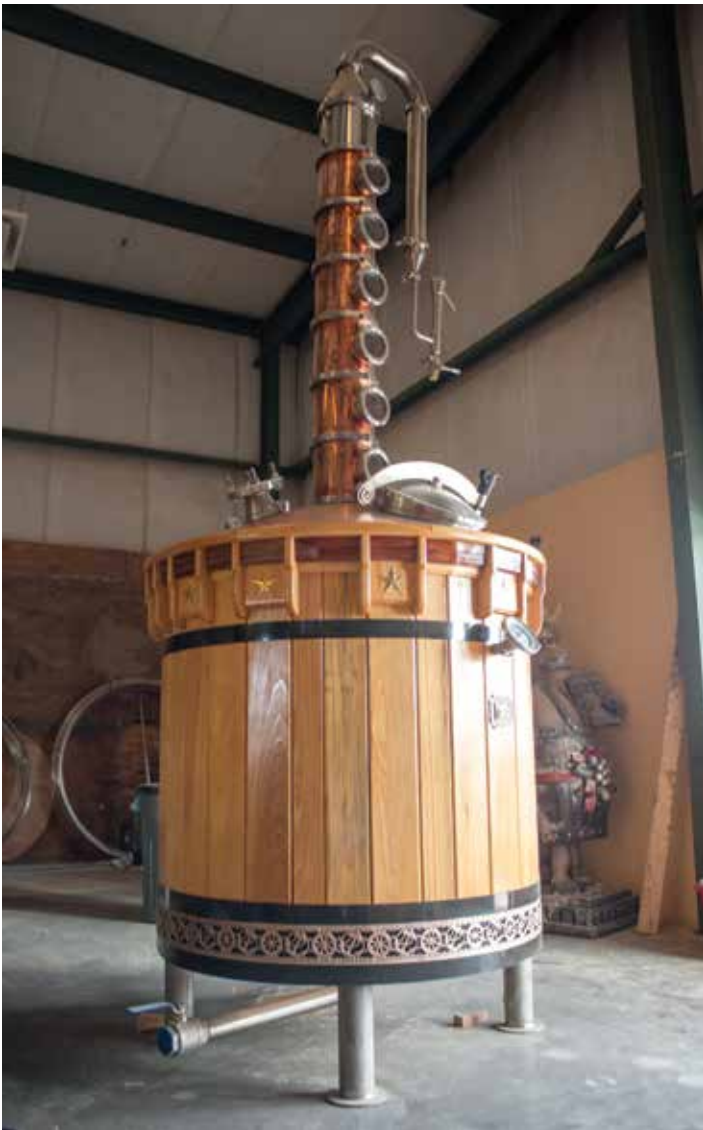
CALDWELL'S STILLS ARE DECKED OUT IN A PATENTED WOOD ENCASING AND CUSTOMIZED FOR EACH DISTILLERY THEY'RE PRODUCED FOR AT CONFEDERATE STILLS OF ALABAMA'S CHILDERSBURG PRODUCTION FACILITY.
