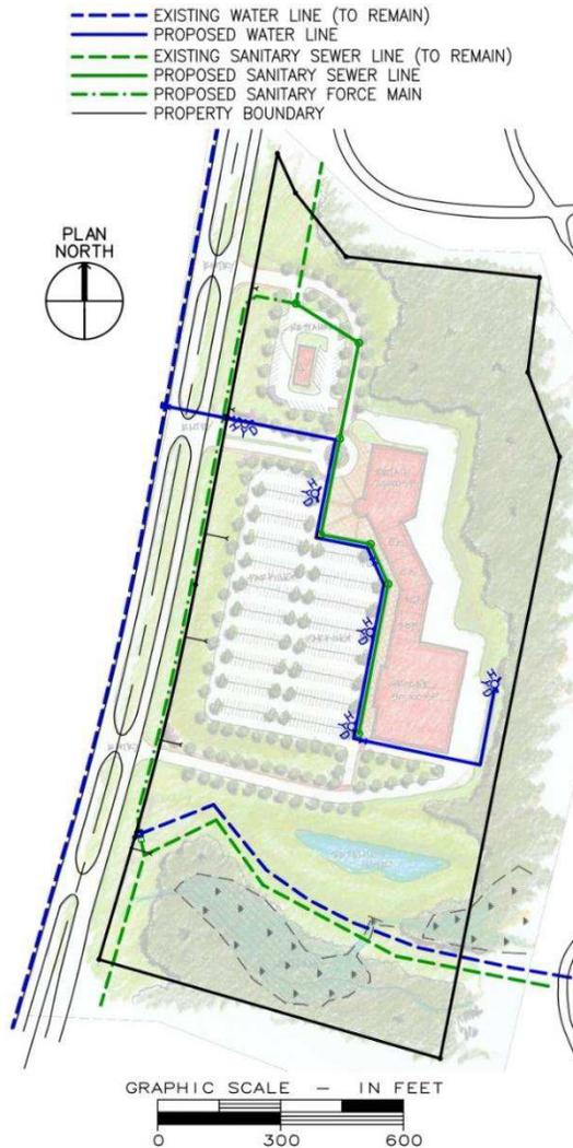
Note: AWWSB existing infrastructure shown. MDA data shows water and sewer lines in the area that are not verified as part of the AWWSB infrastructure and would need to be located and verified prior to design and construction.
