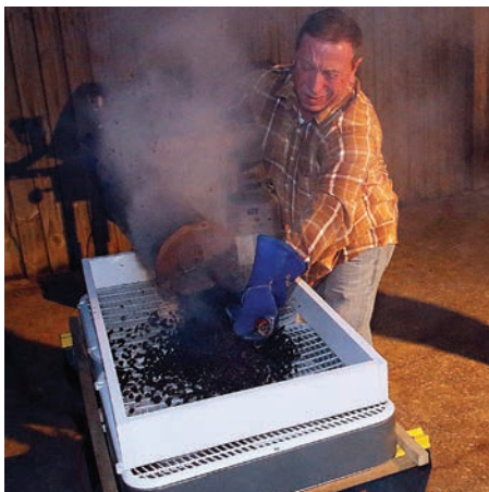
TRANSFER: Jones dumps the freshly roasted coffee beans into a box with a mesh bottom for cooling.
