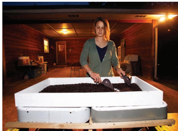
COOL: Sparks stirs the roasted coffee beans in a box with a mesh bottom to help cool the coffee beans. The box is sitting on two box fans that blow air over the hot beans.
