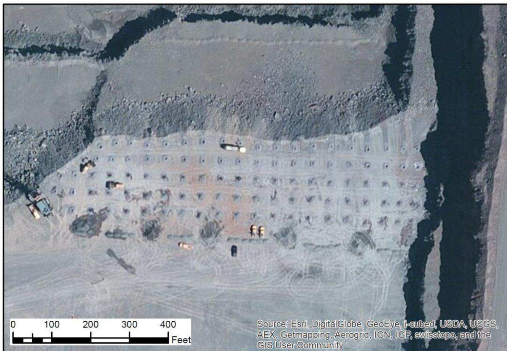
FIGURE 5. DRILLING OPERATIONS IN PREPARATION FOR SURFACE BLASTING AT THE MINNTAC MINE IN MOUNTAIN IRON, MN. THE DRILL RIG IS VISIBLE AT LEFT.
