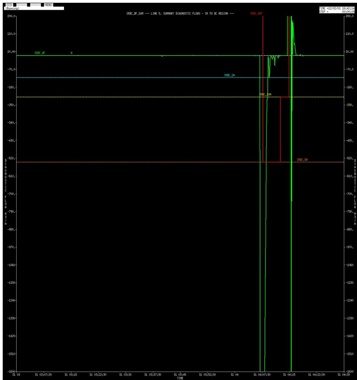
Figure 19: MBS Diagnostic Flow Summary – - NTSB/PHMSA IR 358, Source: Enbridge N0.172945
