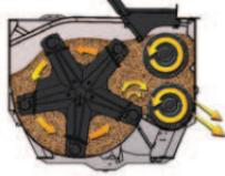
Reel and auger design allows for economical, low fuel consumption
