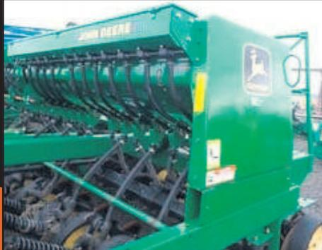
We have gone from end to end on this disk. Rear blades measure 21" and the front 20" All cylinders are dry and all new tires on the center section. Discs are all in great condition as well as harrows.
