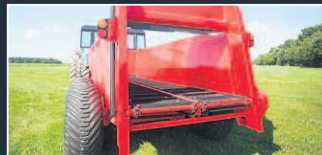
Dual apron provides consistent and reliable material flow to beaters
