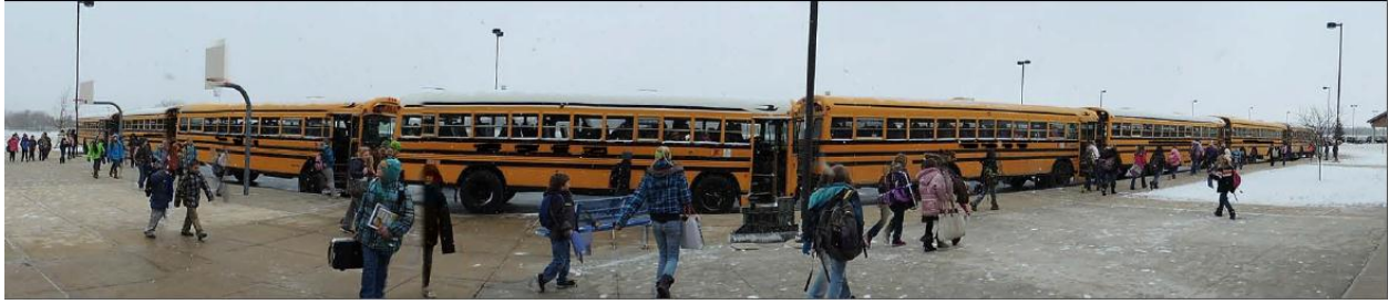
Figure 23: Buses stacked closely, preventing or slowing emergency egress. Sight lines to surrounding areas heavily obscured.
