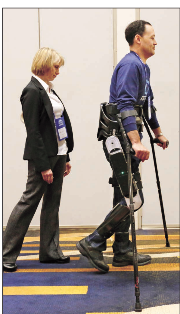
The Associated Press Michael Gore, right, who is paralyzed from a spinal injury, walks with the use of the Indego wearable robot under the supervision of physical therapist Clare Hartigan during a meeting of the American Spinal Injury Association at a downtown hotel in Chicago on Monday.
